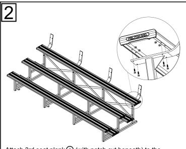
Attach 3rd seat plank (3) (with notch cut beneath) to the assembly in step 1 by using bolts (7) and nuts (8) as illustrated.
