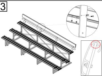
Install the backrest plank 4 onto frame fixing plates as illustrated. Fasten the backrest plank 4 with hexagonal bolts 7 and nuts 8. Ensure the fixing plates are installed in the right place on backrest plank.
