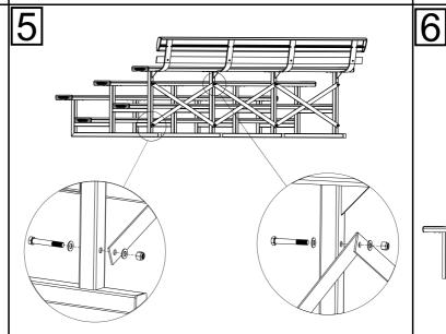
Attach six flat bars ⓑ to the back of base frames ① by using bolts ⑪ , washers ⑫ and nuts ⑬ as illustrated.
