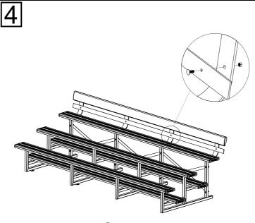
Attach the long flat bar (5) to fixing plates by using bolts (9) and nuts (10) as illustrated.
