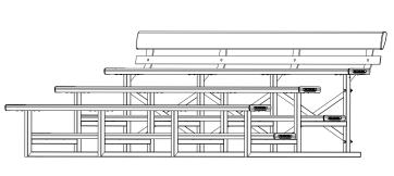
Tighten all hexagonal head bolts with spanners and appropriate tools. Then completely tighten the M12 dynabolts to attach the whole assembly firmly to the ground.
