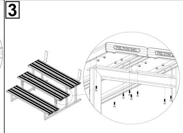
Repeat step 2 with four remaining planks 3 at lower positions on base frame 1
