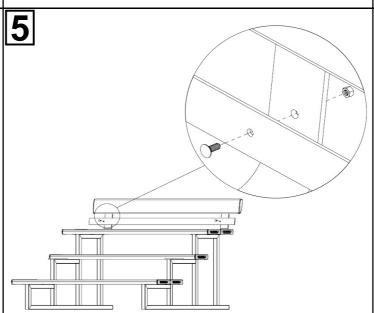
Attach the long flat bar **5** to fixing plates by using bolts **8** and nuts **9** as illustrated.
