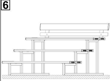
Tighten all hexagonal head bolts with spanners and appropriate tools. Then completely tighten the dynabolts to attach the whole assembly firmly to the ground.
