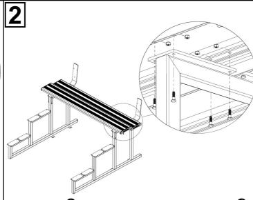
Attach plank **3** to the assembly in step 1 by using bolts **6** and nuts **7** as illustrated.
