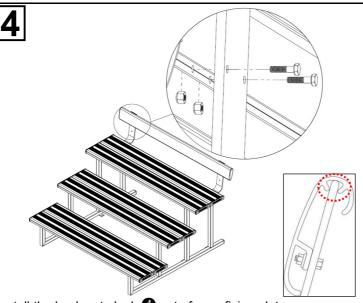
Install the backrest plank **4** onto frame fixing plates as illustrated. Fasten the backrest planks 4 with hexagonal bolts
