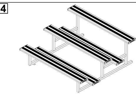
Tighten all hexagonal head bolts 3 and nuts 4 with spanners and appropriate tools. Then attach the whole assembly to the ground by using M12 dyna-bolts preferably, on each frame lug.
