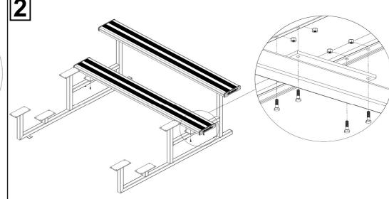
Attach another plank 2 to two base frames 1 at the lower position by using bolts 3 and nuts 4 as illustrated.
