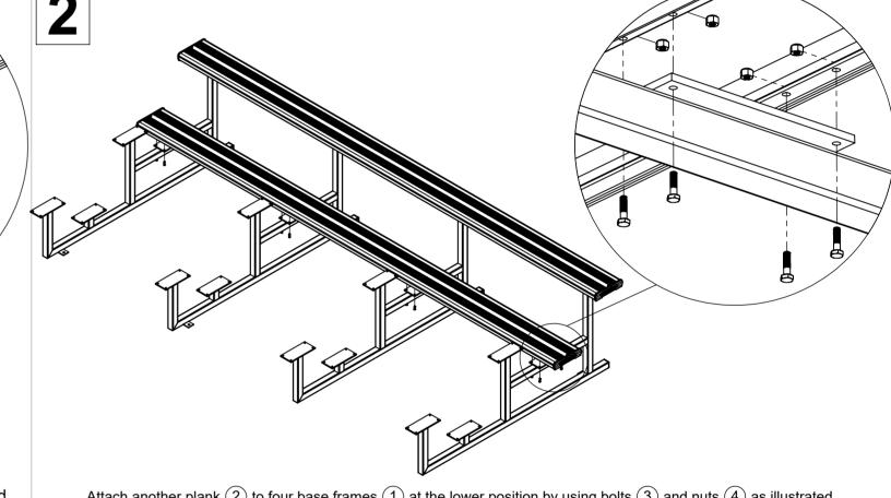
Attach another plank (2) to four base frames (1) at the lower position by using bolts (3) and nuts (4) as illustrated.
